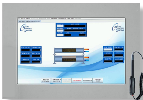
EVAPORATOR CONDENSER OVERVIEW SCREEN
